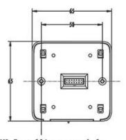
2-M3 Installing screw hole
